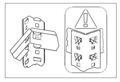
3. Join the two end assemblies together with the long beams (C).
